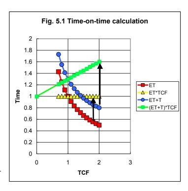
TCF (the green line in Figure 5.1). Therefore the larger the TCF the more extra corrected time is added by the calm period, and the larger boats suffer more than the smaller ones.
