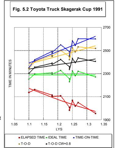
smallest boats do not even manage to finish, when the wind drops completely. Typically in evening races the wind drops and favours the largest boats. One way of compensating for this is to start the larger boats later than the smaller ones, and try to adjust the starting time so the smaller and larger boats finish at the same time.
