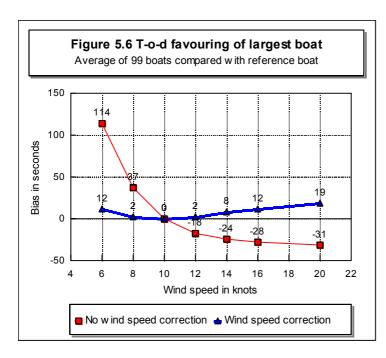
Table 5.3 and Figure 5.6 show that the average favouring for 99 boats as compared to the reference boat IMX-38 is considerably reduced by the application of CW. Table 5.3 also shows that there is a fairly large spread of results. This is due to the fact that heavy and light wind boats come out differently, and that the shapes of the performance curves are slightly different. The standard deviation is also considerably reduced by the application of CW.
