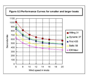
for the period of the race when it was blowing was not average. but it was fairly heavy weather. This illustrates that time-ondistance gives completely wrong results, if the calculation is not corrected for wind speed. There is a widely spread misunderstanding that timeon-distance can be used without such a correction. As soon as the wind speed is below or above the average wind speed for which the rating is valid, time-ondistance gives gross errors.
